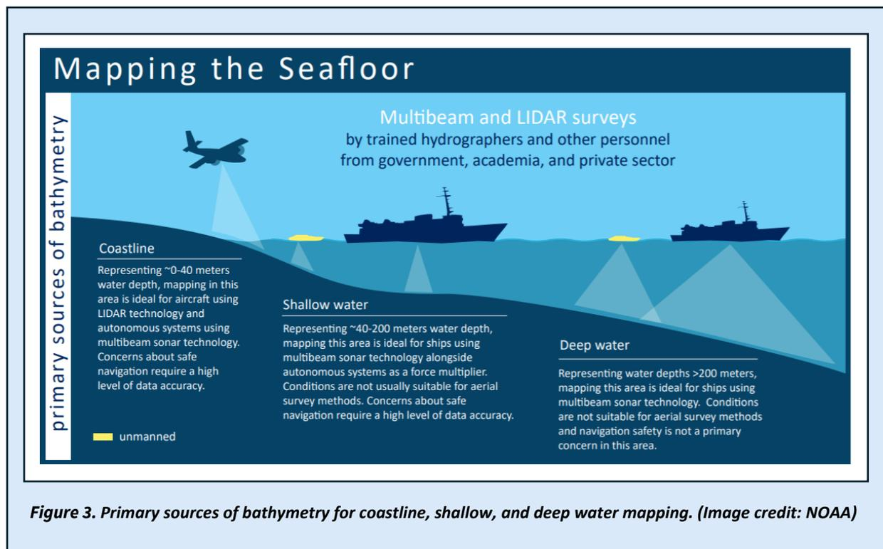
Figure 3. Primary sources of bathymetry for coastline, shallow, and deep water mapping. (Image credit: NOAA)
